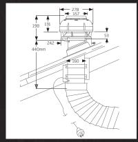
850m<sup>3</sup>/hr - 900m<sup>3</sup>/hr (220 l/s-250 l/s) extraction power
