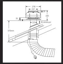
550m<sup>3</sup>/hr - 650m<sup>3</sup>/hr (150 l/s-180 l/s) extraction power
