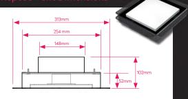
Dimension of Vents: Outer Frame - 315mm x 315mm Diffuser - 200mm x 200mm
