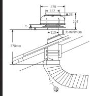
550m³/hr - 650m³/hr (150 l/s-180 l/s) extraction power
