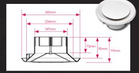
Dimension of Vents: Outer Diameter - 265mm Diffuser Diameter - 185mm
