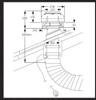
850m³/hr - 900m³/hr (220 l/s-250 l/s) extraction power
